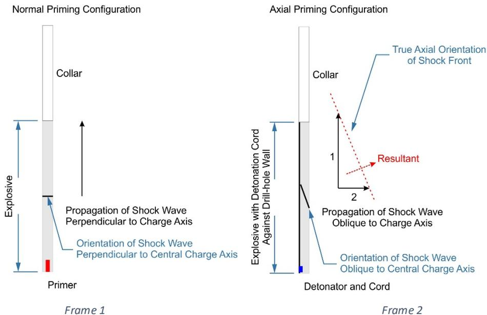
Figure 1 - Normal method of priming an explosive column (Frame 1) vs the axial method of tracing an explosive column (Frame 2).
