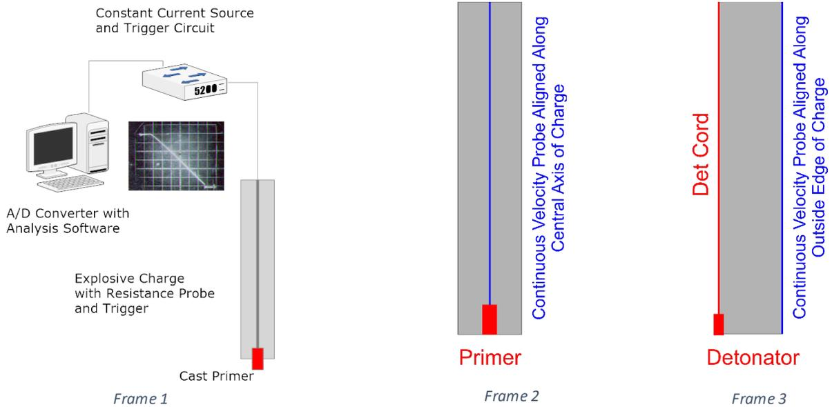
Figure 2 - Method of capturing VoD from an explosive product shown in Frame 1. Normal priming consists of a primer and probe oriented along the central axis of the explosive whereas the position for monitoring the VoD for an axially traced charge is shown in frame 3. The shock wave generated would be oblique.
