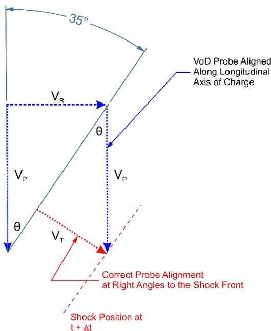
Figure 7 - Velocity vectors associated with axial initiation showing the resultant shock front. It should be noted that the detonation velocity should be measured perpendicular to the resultant.  $V_R$  is the radial velocity of the cord sensitive explosive charge and  $V_P$  is the detonation velocity of the detonating cord.
