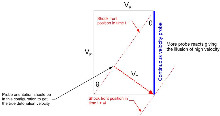
Figure 6 - Priming shock wave orientation diagram showing the orientation of the shock wave (red) with respect to the VoD probe (blue). This unit charge is based on velocity vectors for both primacord and an emulsion. It is easily seen that the continuous velocity probe is oriented in the wrong direction and will always give higher VoD readings.
