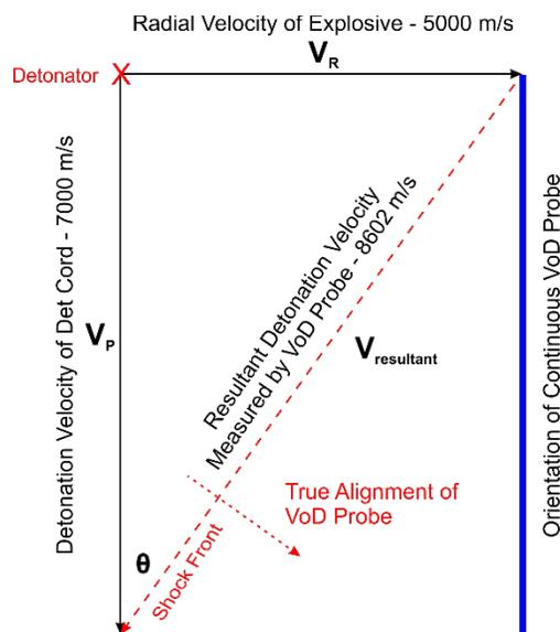
Figure 4 - Shows velocity vectors for the axial orientation of detonating cord and with reference to the radial velocity of a typical emulsion explosive. These are drawn to scale (cord velocity – 7000 m/s with 5000 m/s for explosive velocity with no run-up). It can be shown that the continuous velocity probe will read 8602 m/s because of the probe's alignment. More probe will be reacted per unit time in the configuration shown than a probe aligned perpendicular to the shock front.
